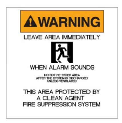
Exit Warning Sign, this is to be located at the door inside the protected room.
