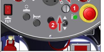
To start the machine, turn the key (1) set the direction switch to forward (2) set the speed control and water flow rate(3).
