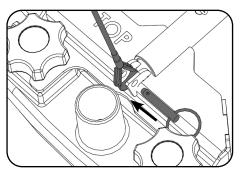
Fit the floor tool and retain using the detent pins.
