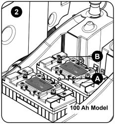
Your machine has been designed to work at the optium brush pressure with a weight set added into the 50 Ah model in place of an additional battery 100 Ah model.
