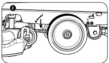
The machine is equipped with a free-wheel function that will enable the operator to move the machine manually if required. The motor brake is located on the right side of the machine near the rear wheel. Lift the Arm to the upper position for Drive (Fig.1). Lower the arm to disengage the drive (Fig.2).
