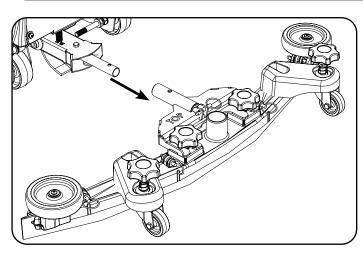
To clean the floor tool, remove securing-pin and pull-free from the holder.
