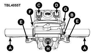
TBL4055T models only set direction of travel (F) and the desired traction speed as required (G), depending on floor type and level of soiling. Middle speed is the optimum cleaning speed.
