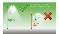
A spot lamp unit mounted near to an EXIT sign would almost certainly cause sufficient glare to make the EXIT sign illegible.
