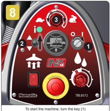
set the direction switch to forward (2) set the speed control (3).
