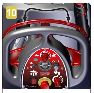
Pull the start triggers with the deck down, this will start the brush spinning.
