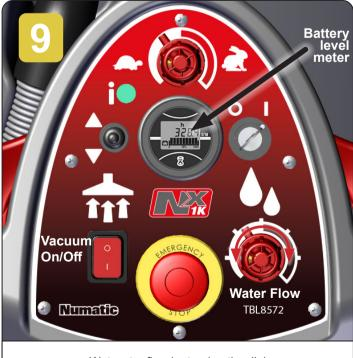
Wet water flow by turning the dial and the Vacuum On/Off button as required.
