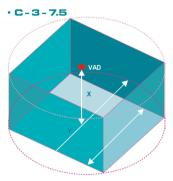
A ceiling mounted VAD uses a similar rating formula, with two numbers representing the coverage volume, this time in the shape of a cylinder, where the first number is the maximum ceiling height to which the VAD can be mounted, and the second number is the diameter of the coverage.
