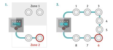
**1. Conventional** - A conventional fire detection system employs 'spurs' of detectors grouped into Zones. When a detector is in alarm/fault only the Zone is reported at the CIE.
