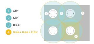
For heat detectors, individual detector coverage is **5.3m** radius, but again, because these radii must overlap, the actual distance between the detector and the wall must be **3.8m** and between detectors must be **7.5m**.
