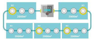
**Short Circuit Isolators** (either on the loop or within the CIE) should be installed to limit the loss of fire cover caused by a single fault to 2000m<sup>2</sup>
