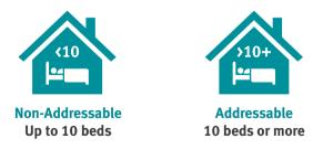
Where occupants of a building are going to need assistance from staff to evacuate the building (e.g. in residential care premises and hospitals), the fire detection and fire alarm system should be ADDRESSABLE if the building has facilities for MORE THAN 10 PEOPLE to sleep..
