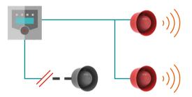
Alarm Device Circuits (should be arranged so that, in the event of a single fault, at least one sounder, sited within the vicinity of the CIE, will continue to operate.
