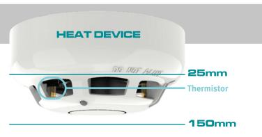
The minimum static response of heat devices should not be less than 29°C above the average ambient temperature, or less than 4°C above the highest temperature the device can be expected to experience.
