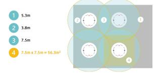
An important note on multi sensors that can operate as either smoke or heat. According to BS5839-1 these have to be spaced as per the heat spacings previously, even if they are installed as smoke-only. This is to future-proof the installation against possible change of use or new/updated risk assessments.
