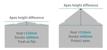
For ceilings that feature an apex: as long as the height difference between the apex and the height of the eaves is less than 150mm for Heat detectors or less than 600mm for Smoke detectors then these can be treated the same as flat ceilings.
