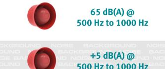
Sufficient sounders, operating within the frequency range of 500 Hz to 1000 Hz, should be installed to endure that a sound pressure of 65 dB(A). Add 5 dB(A) above a background noise (if lasting more than 30 seconds) at all accessible points will all doors closed.
