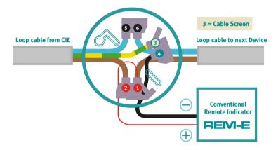
All remote indicators should be tested at least once per year and should be wired with the same grade of cable as the detection circuits (Enhanced/-Standard). This can be reduced to 1mm<sup>2</sup> to facilitate installation.
