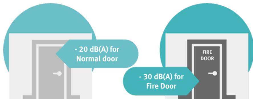
A reduction in sound pressure of approximately **20 dB(A)** may be expected through a normal door, and approximately **30 dB(A)** through a fire door.
