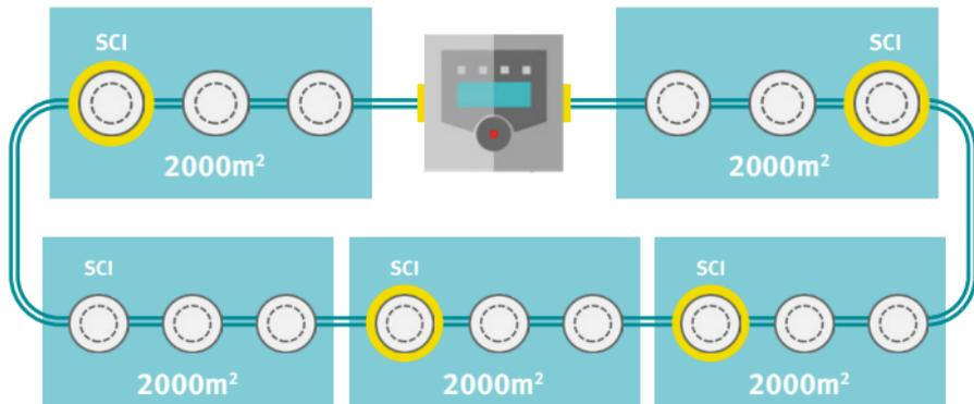
**Short Circuit Isolators** (either on the loop or within the CIE) should be installed to limit the loss of fire cover caused by a single fault to **2000m<sup>2</sup>**
