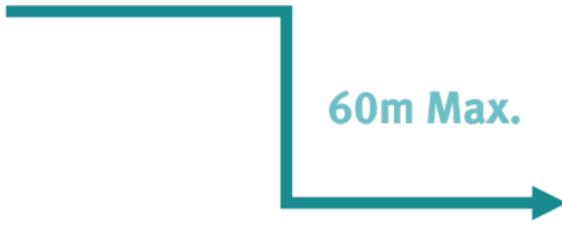
A person searching a Conventional Zone for a fire should not have to travel more than **60m** from the point of entry into the Zone to identify evidence of a fire.
