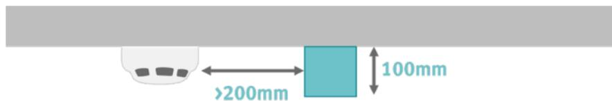
**If a ceiling obstruction is less than 250mm, or less than 10%** of the ceiling height, such as a strip light fitting, then detection devices should not be mounted closer than **twice the depth of that obstruction.**
