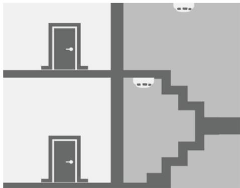
Enclosed stairways should have a detector at the top and at each main landing.
