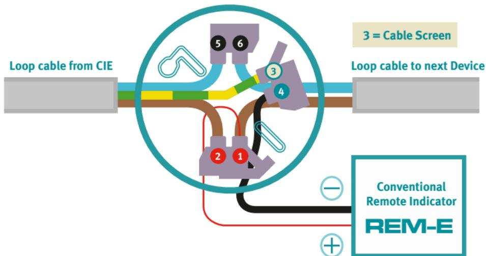
All remote indicators should be tested at least once per year and should be wired with the same grade of cable as the detection circuits (Enhanced/-Standard). This can be reduced to 1mm<sup>2</sup> to facilitate installation.
