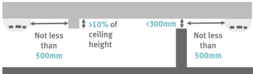
**Ceiling obstructions, if deeper than 10%** of the ceiling height, or floor mounted obstructions (e.g partitions) where the top is less than 300 mm from ceiling should be treated as walls
