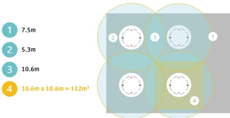
For heat detectors, individual detector coverage is **5.3m** radius, but again, because these radii must overlap, the actual distance between the detector and the wall must be **3.8m** and between detectors must be **7.5m**.
