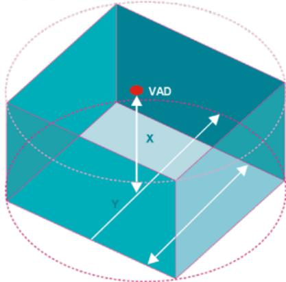
A ceiling mounted VAD uses a similar rating formula, with two numbers representing the coverage volume, this time in the shape of a cylinder, where the first number is the maximum ceiling height to which the VAD can be mounted, and the second number is the diameter of the coverage.
