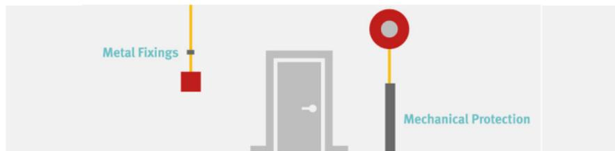
All fire alarm cables, below the height of **2m** from the finished floor level should be mechanically protected, unless enhanced cable is used.
