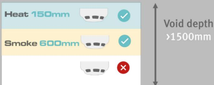
Voids deeper than 1500mm may be treated as a room when siting detectors below the ceiling - 150mm for heat and 600mm for smoke.
