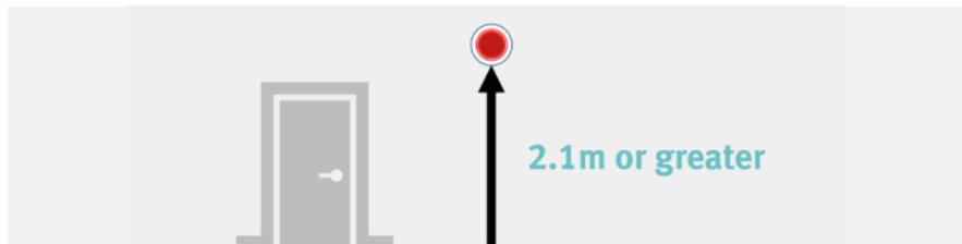
**Visual Alarm Devices (VADs)** such as strobes and beacons may be ceiling or wall mounted, but for wall mounting the minimum of **2.1m** from finished floor levels applies.
