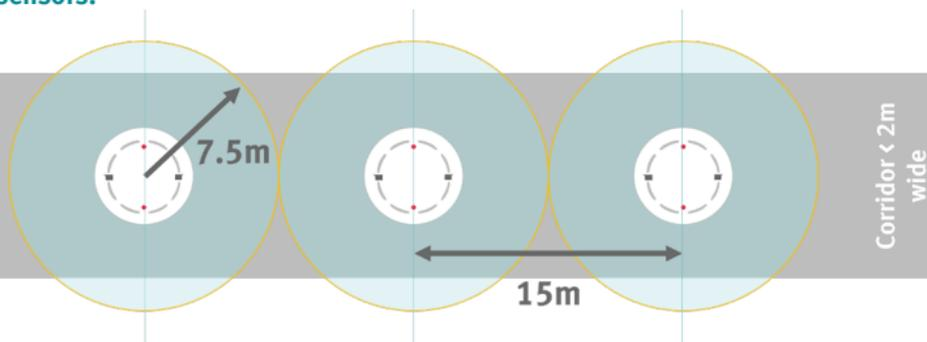
The standard does not recommend using heat sensors in escape routes, unless covered by a variation.
