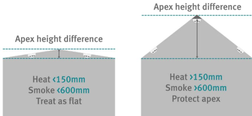
For ceilings that feature an apex: as long as the height difference between the apex and the height of the eaves is less than 150mm for Heat detectors or less than 600mm for Smoke detectors then these can be treated the same as flat ceilings.
