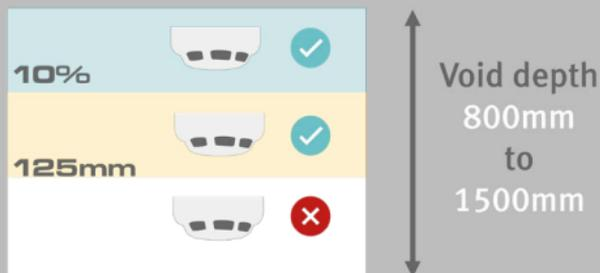
If the system category requires detection in any area, which has a void **deeper than 800mm but less than 1500mm depth**, detection should be provided in the void.
