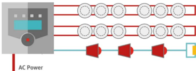
Cables used for the **Critical Signal Path** and the final LV (low voltage) mains supply to any fire detection equipment are now required to be fire resistant and coloured externally in a single, common colour (red is preferred).
