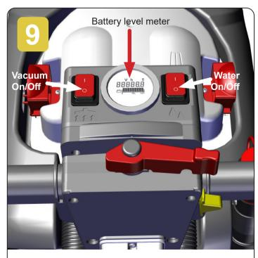
With the machine running press the Water On/Off button and the Vacuum On/Off button as required.
