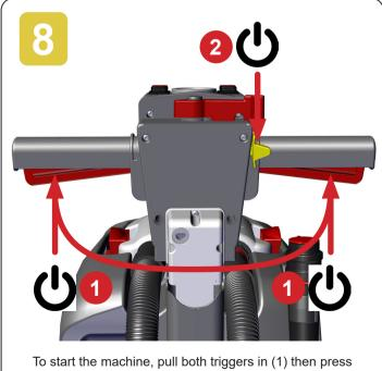
down the start button (2) with the deck down, this will start the brush spinning.
