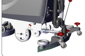
To start the machine, pull both triggers in (1) then press down the start button (2) with the deck down, this will start the brush spinning.
