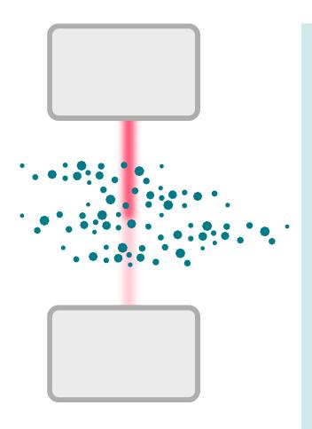
Beam detectors use an obscuration technique, whereby a constant beam of infra-red light is monitored for a decrease in strength due to smoke particles obscuring the beam. They can cover a huge volume of space and therefore are often used in leisure centres, shopping centres and auditoriums etc.
