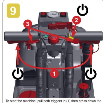
start button (2) with the deck down, this will start the brush spinning.
