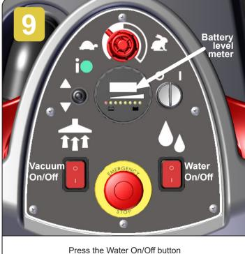
Press the Water On/Off button and the Vacuum On/Off button as required.
