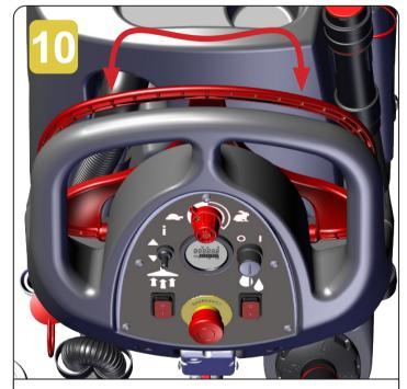
Pull the start triggers (2) with the deck down, this will start the brush spinning.
