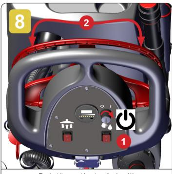
To start the machine, turn the key (1) then pull the start triggers (2) with the deck down, this will start the brush spinning.
