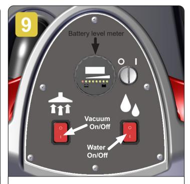
With the machine running press the Water On/Off button and the Vacuum On/Off button as required.
