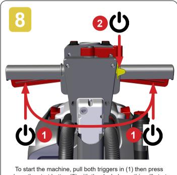
down the start button (2) with the deck down, this will start the brush spinning.
