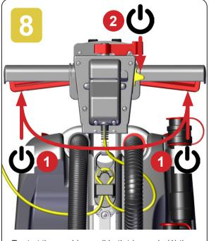
To start the machine, pull both triggers in (1) then press down the start button (2) with the deck down, this will start the brush spinning.
