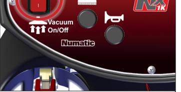
With the machine running press Vacuum On/Off button
