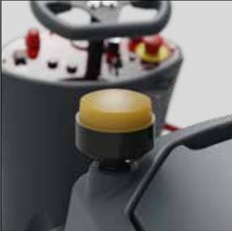
On-board safety features: emergency stop, horn, power-off key and hazard warning light.
