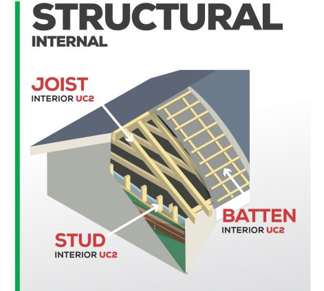
For wood in permanent ground or fresh water contact, or providing exterior structural support, Use Class 4 levels of protection MUST be achieved. Anything less and service life, structural safety and customer satisfaction will be compromised.
